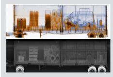
The Eagle M60 ZBx produces two X-ray images in a single scan: a high-energy transmission image and a Z Backscatter image.
